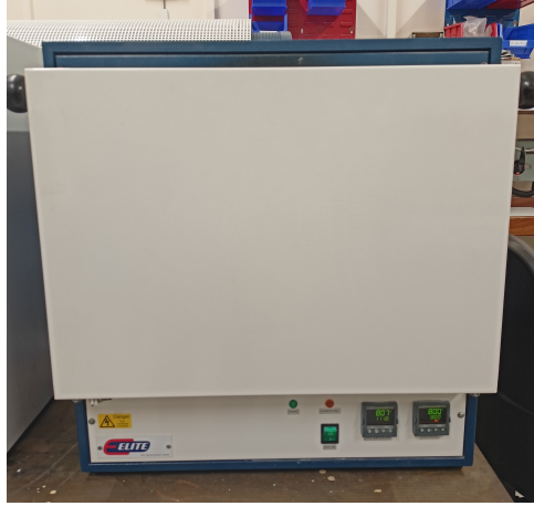
FIGURE 2.3: The three-zone furnace used for growing the single crystal samples. It had a temperature gradient due to the leakage of heat through the furnace door, which allowed for the horizontal Bridgman technique to be used for the synthesis. The heating run could be automatically controlled using the interface on the bottom right of the furnace.
