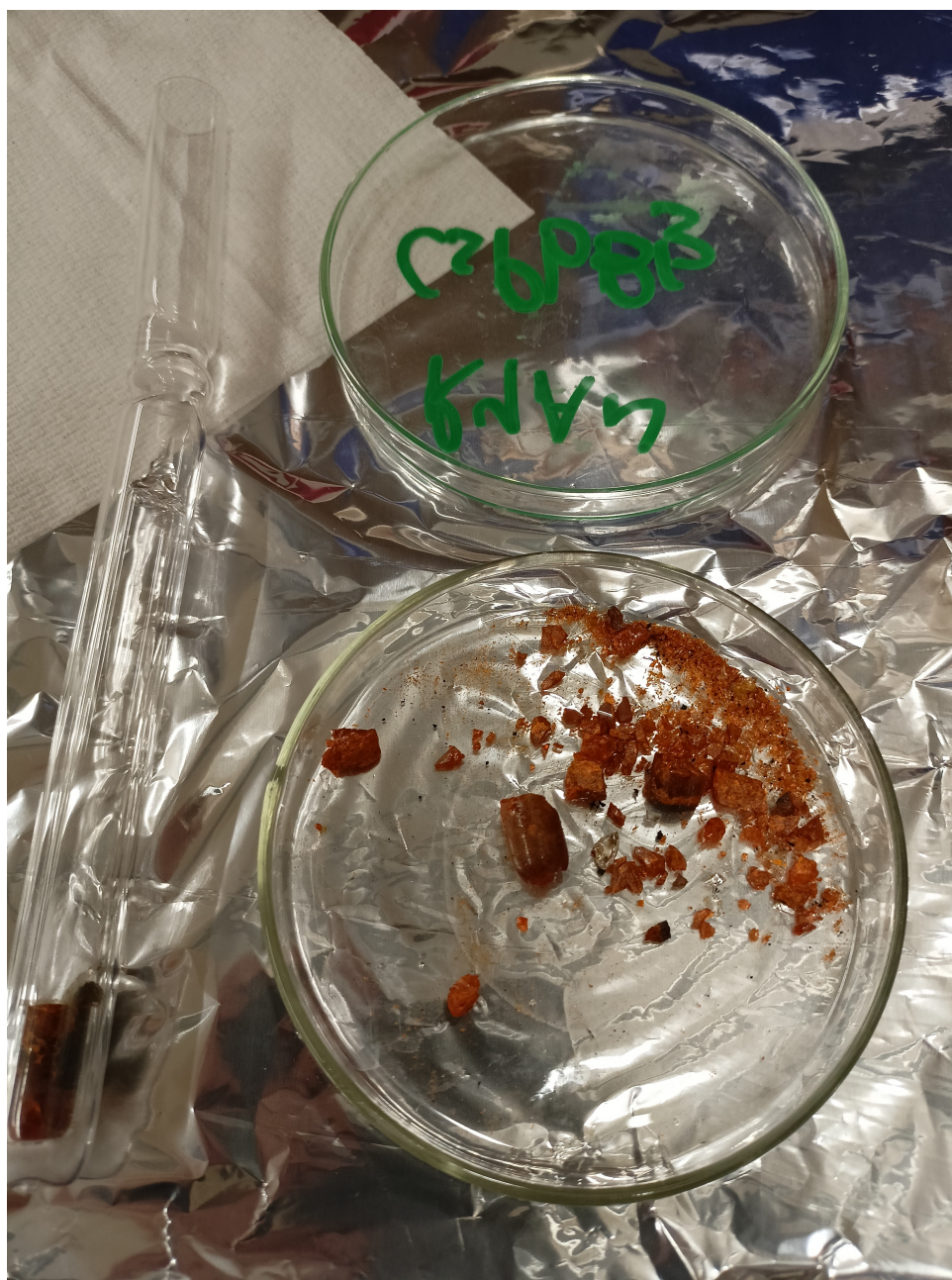
FIGURE 2.8: The \text{CsPbBr}_3 samples produced via the horizontal Bridgman technique that used the relatively uncontrolled environment of the furnace to generate a sufficient temperature gradient in order to cause localised undercooling of the stoichiometric melt in a crucible.
